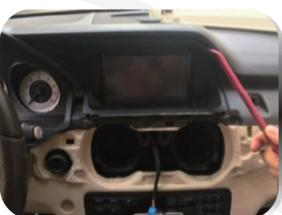
6. Carefully pry and remove the frame of the OEM screen.
