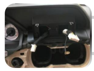
11. Assemble the Android stand securely on the dashboard and ensure that the cables are routed properly.
