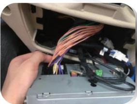
10. Disconnect the power harness from the NTG unit and connect it to the Android harness. Please refer to page 7 for the wiring diagram.
