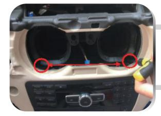
8. Loosen the left and right fixing screws of the NTG Unit.
