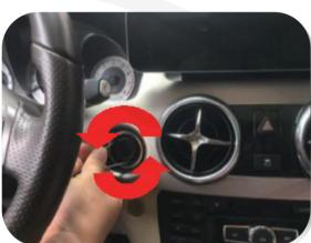
2. Use a tweezer to rotate the silver ring in a counterclockwise direction.
