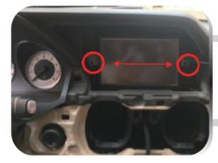
7. Remove the left and right fixing screws of the OEM screen and take out the panel.
