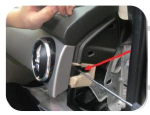
4. Remove the side fixing screws from the air conditioning port.
